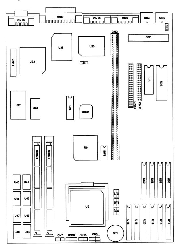
System board components and connectors
